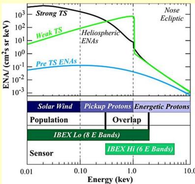
[Above] An example of expected ENA fluxes for strong and weak termination shocks. The IBEX Hi and Lo sensors overlap and compliment each other to provide the best coverage of the energy spectrum.
