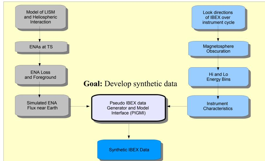
[Above] Physics and model variables (left) are combined with mission parameters (right) in PIGMI to create count rates similar to what IBEX will encounter. This artificial data is providing insight on how to fine tune the data collection process as well as how to standardize the interface between models and IBEX data. The interface will give researchers the tools to readily interact between data and model as the data is provided from IBEX.
